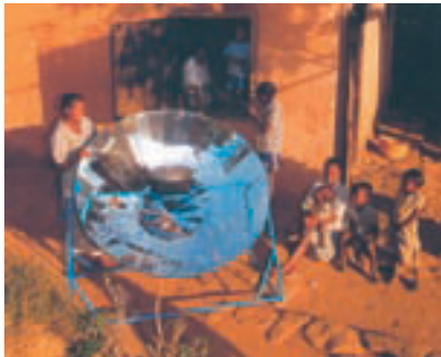
↓ The solar cooker, increasingly in use in developing countries, concentrates the sun's rays to cook food. An economical system, it functions both as an oven and a hotplate. www.solarcooking.org
