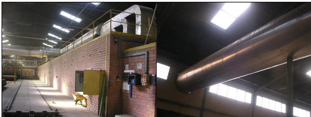
Image 7.3: Using gases from the firing kiln
