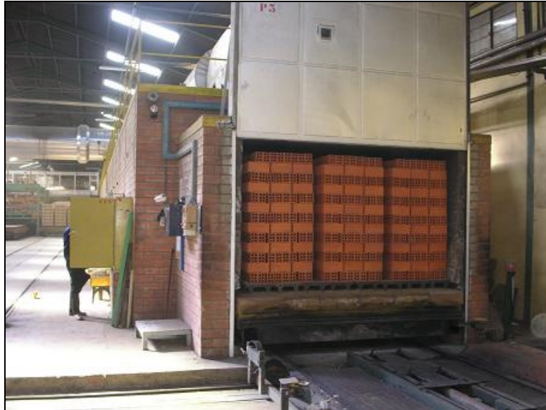
Image 3.9: Tunnel kiln, output material after the firing process
