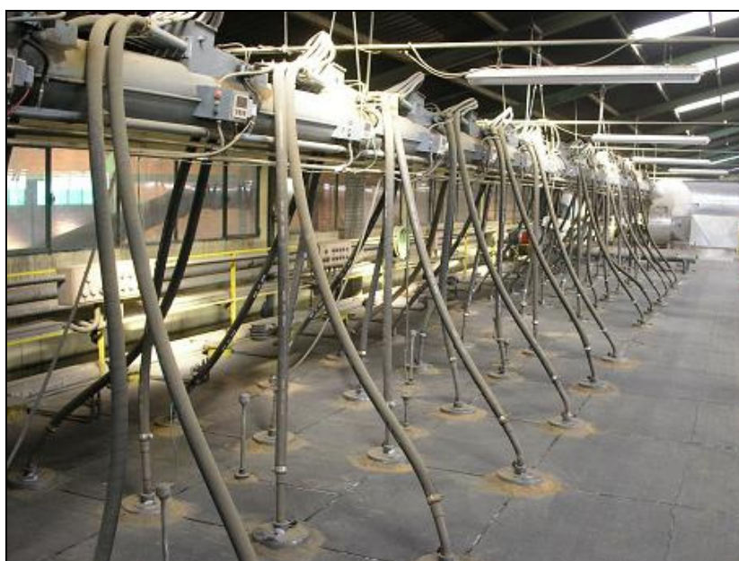
Image 2.2: Ceramics kiln with mixed feed burners of fuel oil and micronised coke
