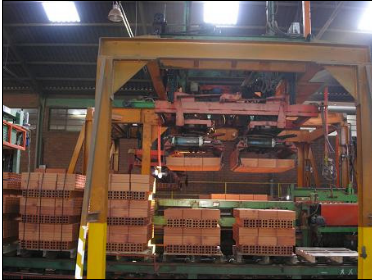
Image 3.10: Stacking the material for its subsequent shrink-wrapping
