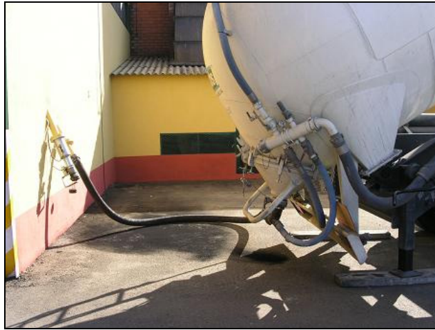
Image 7.1: Supply of petroleum coke to the installation
