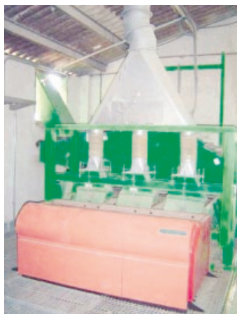
Machine to separate the glass contained within the glass recycling refuse
