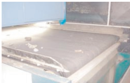
Machine vision unit for separating metals contained in banal waste
