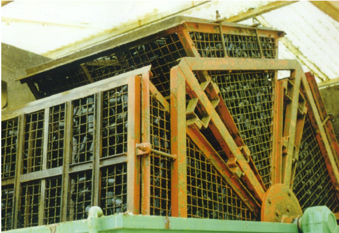
Bio-wheel system to transform vegetable water into a liquid with fertilisation properties (Romanos, Messinia, Greece)
