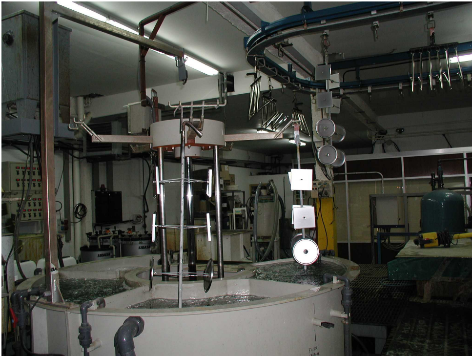
2 - Automated washing installation with programmable robot.
