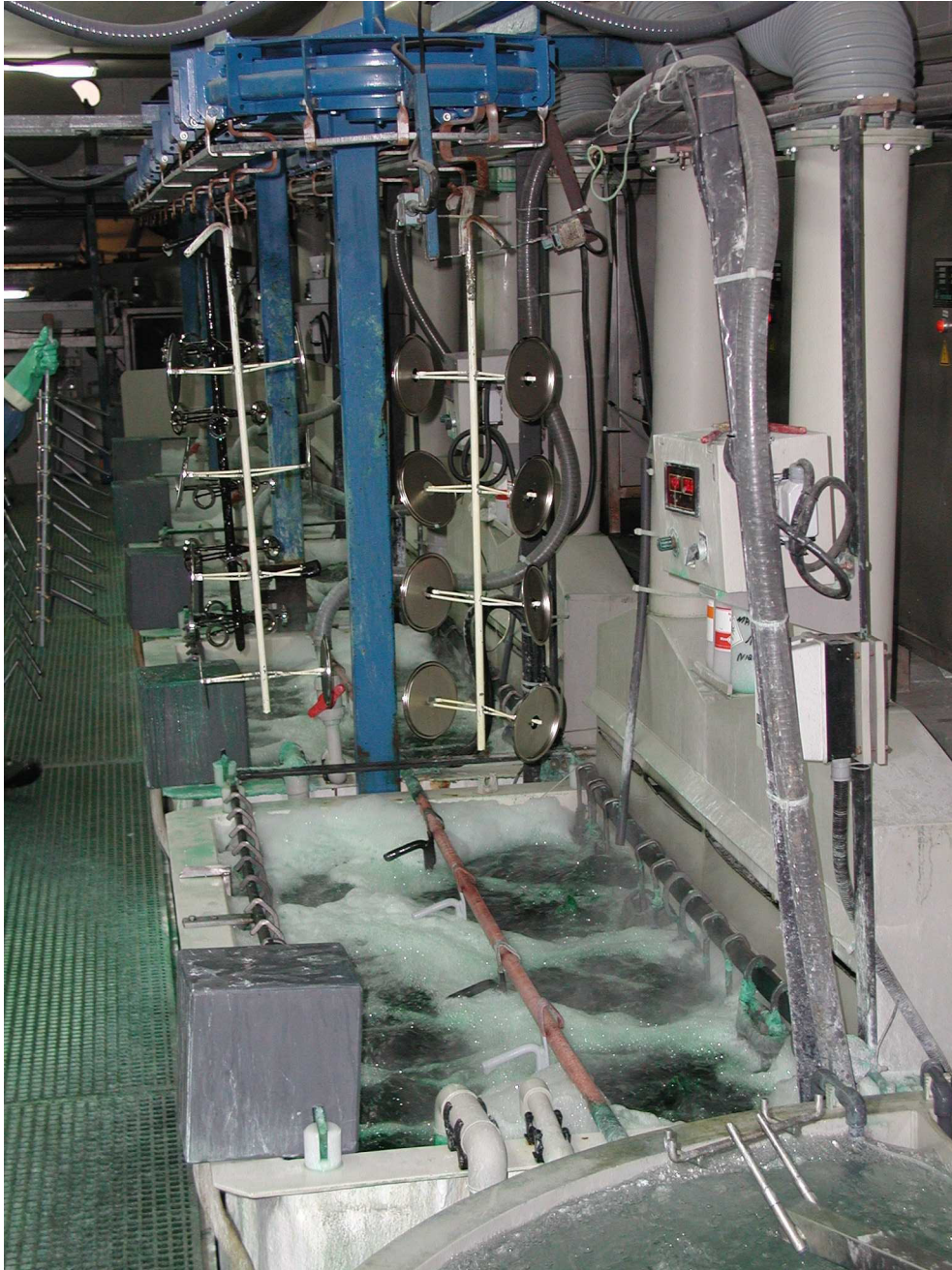
11 – Fume extraction systems for the nickel baths.
