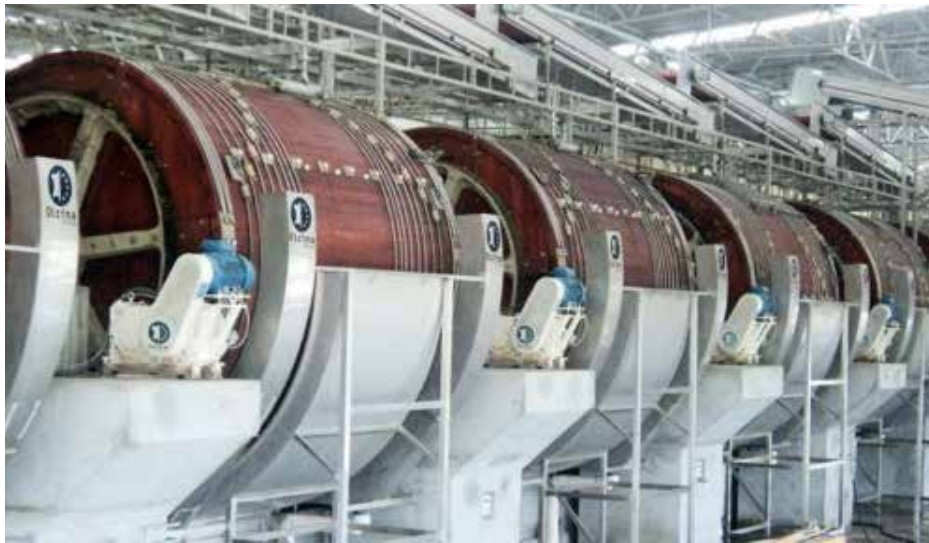
Figure 1. Olcina latest technology Cangilones Next Drums Ø 4.2x4.5m. (Picture courtesy of Gruppo Mastrotto - Italy)
