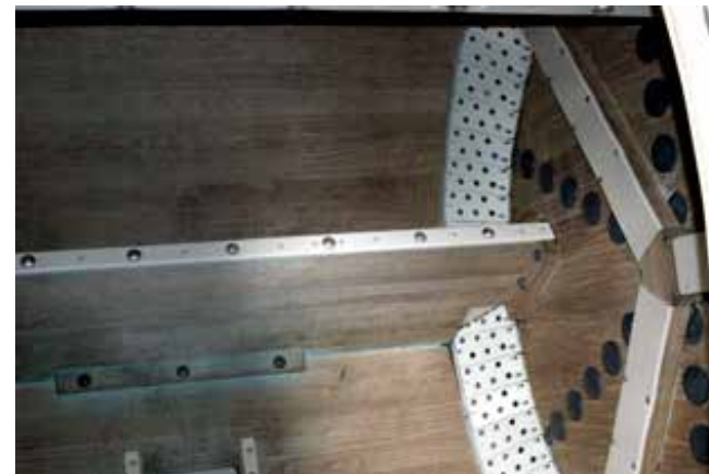
Fig 3: Cangilones off-centre shelves (not looking to the axle) enable hides and float to be lifted to the highest level inside the drum before dropping this mass on top of other hides, creating the «sponge effect».
